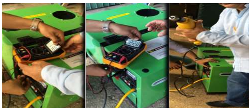
Figure 7. Generation of electric energy. (a) 110 V; (b) 220 V; (c) Using a power drill.
